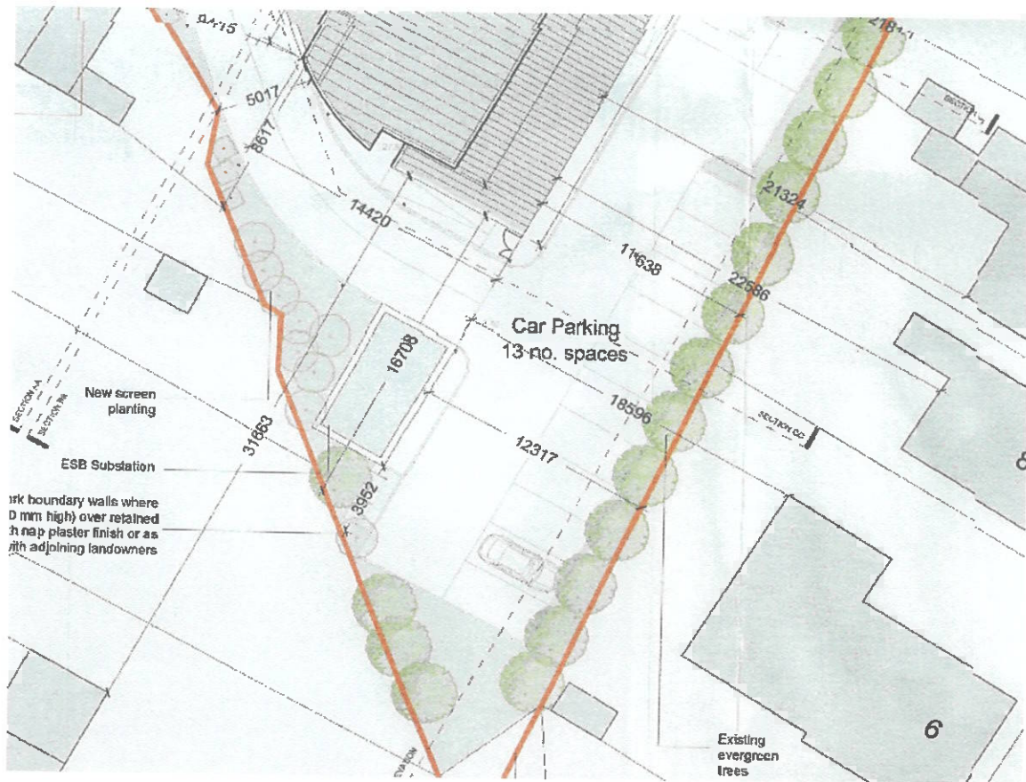
FIGURE (i) Extract from Site Layout Map (Drawing No. W: 16 JOBS P-S-250A lodged with reply to Further Information on 4 th of July 2017. It shows the car park 13 spaces required. It shows the dimensions of the ESB Substation from the Boundary wall and the house of No. 6 Forster Court.
